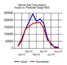
In all, PVNCCDSB has lowered its energy intensity from 2011 to 2012 indicating a slight degradation in energy utilization from  $0.56 \text{ GJ/m}^2$  to  $0.61 \text{ GJ/m}^2$ . Current consumption patterns are tracking reasonably well with the baseline performance.
